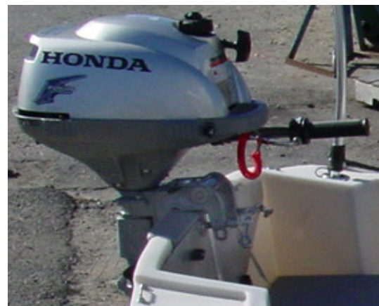
Motor, mounted in place. Note, more recent motor mount plate has side flanges. See preceding photo.
