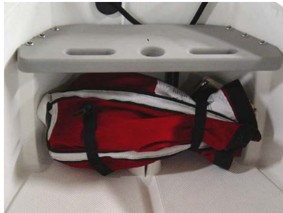
Para-anchor stowed under front (bow) seat
