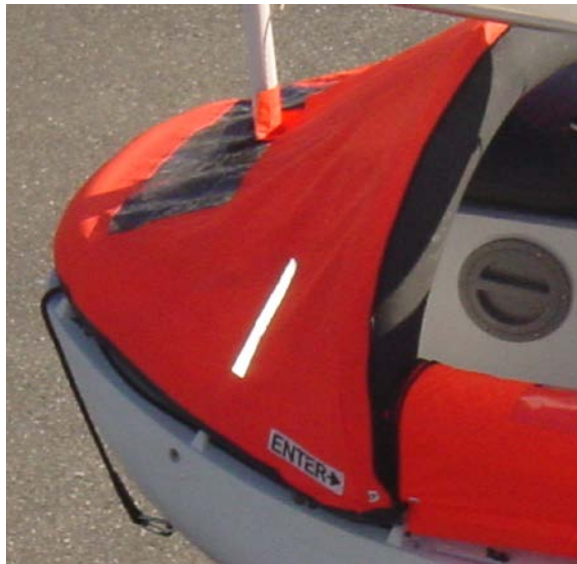
Fore section, showing window, and flap for mast
