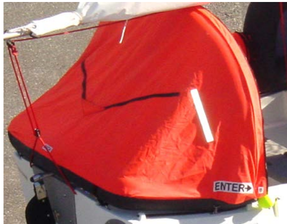
Aft section, Showing Rainwater Catchment
