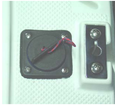
Pump Hatch, Closed
