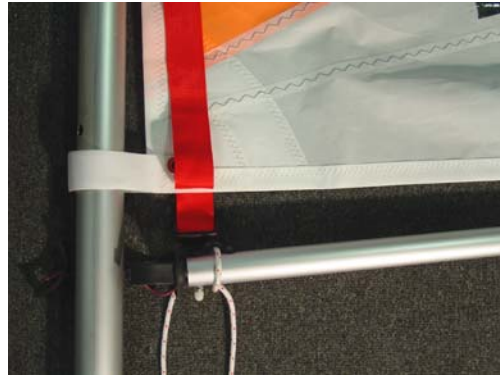
Step E-2. Detail: Detach webbing and buckle from boom.
