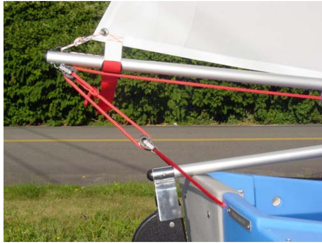
Step H, completed. Traveler installed on boat
