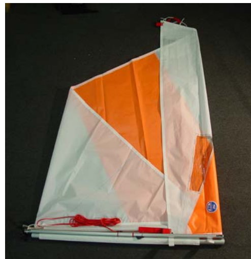
Step E-4. Fold Sail down at peak and up at foot
