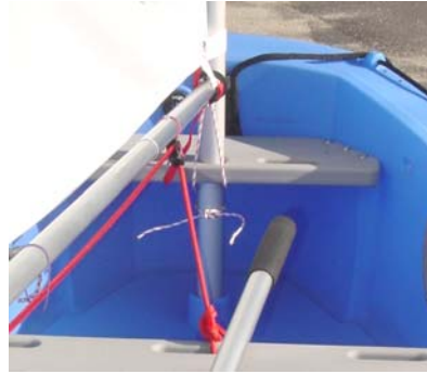
Step G. Mast installed in boat
