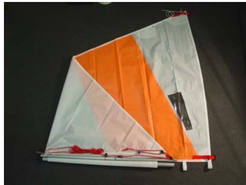
Step E-3. Fold boom up alongside mast
