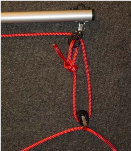
Step H-2. Pass traveler through U-shaped shackle on mainsheet block
