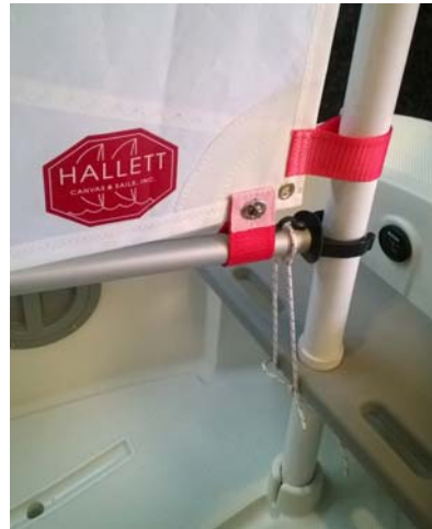
Step G-5. Downhaul passed through the boom's pad-eye. Boom snapped to mast
