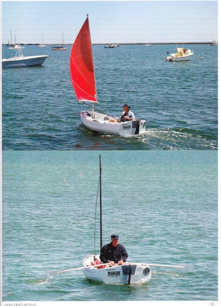
boat made her feel perfectly safe. The Pudgy is self bailing when unloaded. Pulling the plug while not in use keeps bailing to a minimum. While the boat is not selfbailing, I have never taken on more than a slight amount of water. She does float with the plug out even while loaded, although there's a foot and a half of water in the bottom." Kyle Webb, 2007 and 2012 models.
