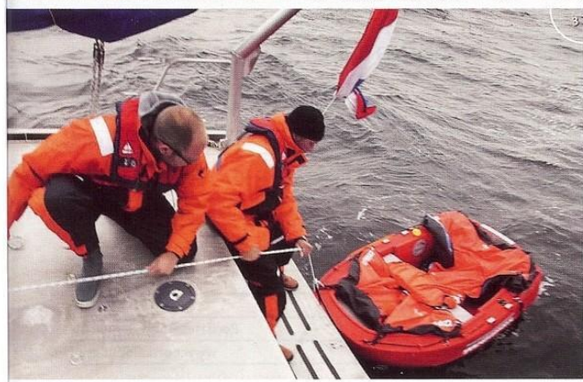
The Pudgy is ready for use on the aft deck of the mother ship. With the cover off we can go overboard. After some pushing and pulling, the Pudgy floats. Under sail there is room for two.
