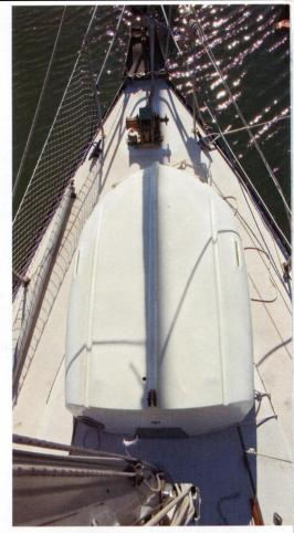
Even though their boat is 40 feet long, the Kinneys' dinghy could not be longer than 8½ feet. At 7½ feet, the Portland Pudgy leaves a little space for working the windlass and headsails, above. At 128 pounds, Pudgy is too heavy to launch and retrieve by hand over the lifelines, but using a halyard and bridle, it's easily raised with a winch, below.
